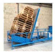
Some costumers find our <u>PalletTipper</u> to big and to expensive. Therefore we developed a smaller PalletTipper. This PalletTipper Type T provides pallets on table height. The PalletTipper Type T is cheaper because the pallets are not automatically pushes forward.
